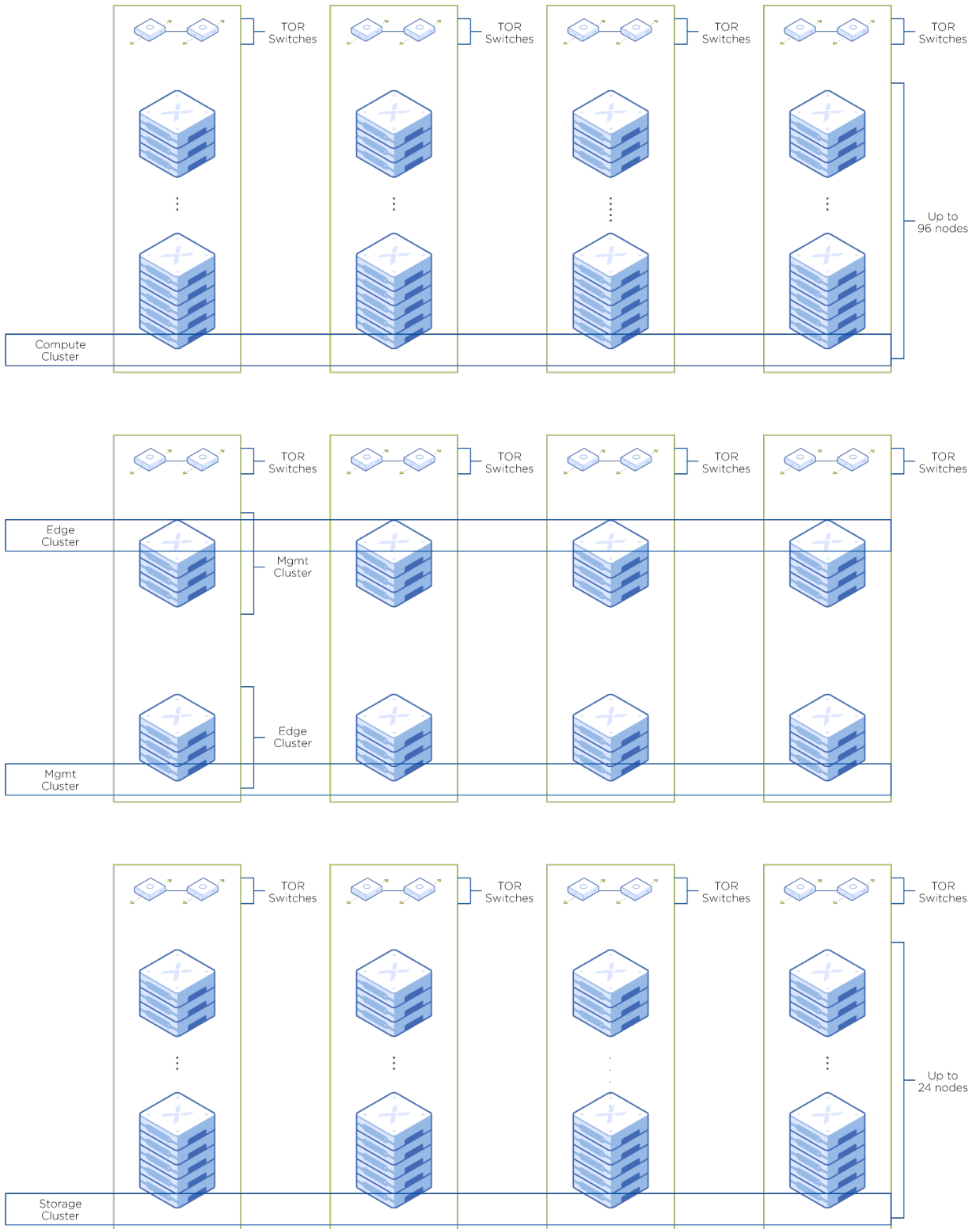
Figure 30: Multiple Racks, Single Workload Domain
